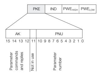
Parameter commands and replies (AK) Bits no. 12-15 are used for transferring parameter commands from master to slave and the slave's processed reply back to the master.
