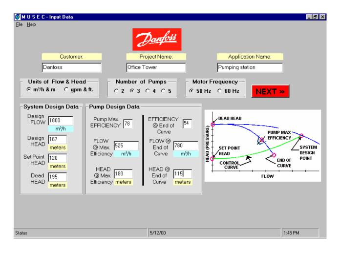
Input scheme with pump and system data
