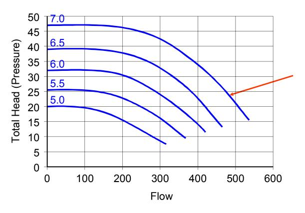
Lines of different impeller diameters
