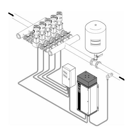
The system consists of 1 variable speed and up to 4 fixed speed pumps/fans
