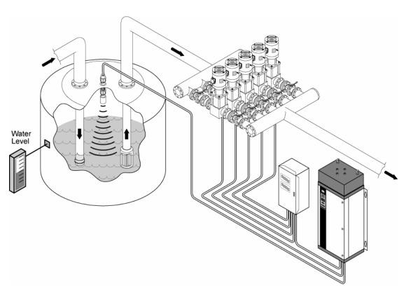
Using the built-in PID controller allows easy inverse control
