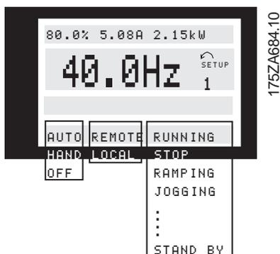
The left indicator on the status line displays the active control mode of the VLT drive. AUTO is displayed when control is via the control terminals. HAND indicates that control is local via the keys on the LCP. OFF indicates that the drive ignores all control commands and will not run.
