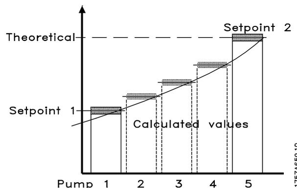
The range is determined by Quick Menu item 14 (parameter 413, *Minimum Feedback*) and Quick Menu item 15 (parameter 414, *Maximum Feedback*). When the pressure feedback signal originates at the far end of the system, the drive does not need to compensate for system pressure changes due to flow. For this system configuration, or for two setpoint PID control, see *Alternative Programming* at the end of this chapter.
