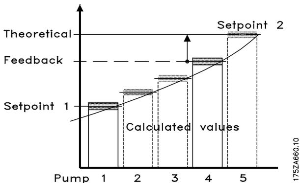
The range is determined by Quick Menu item 14 (parameter 413, *Minimum Feedback*) and Quick Menu item 15 (parameter 414, *Maximum Feedback*).
