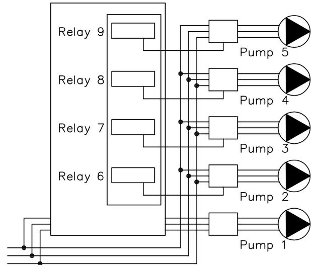
Standard Cascade Controller Setup
