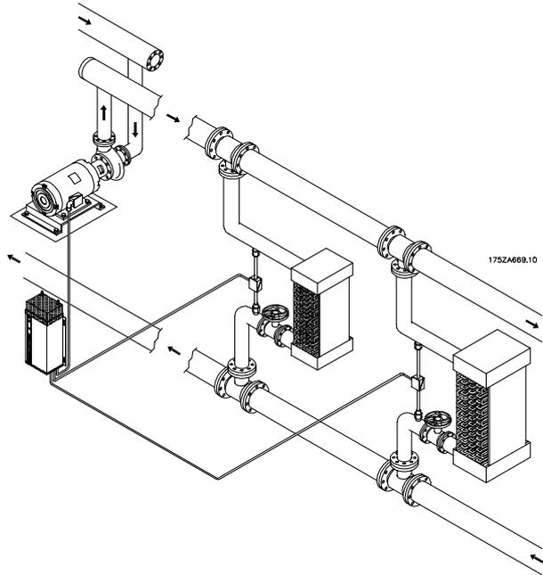
To enable this setup, the feedback function in parameter 417, *Feedback Function*, is selected. When selecting *2-zone Minimum* in parameter 417, the drive will regulate the system so the feedbacks are equal to or greater than their associated setpoints. If *2-zone Maximum* is selected, the feedbacks will be equal to or less than their associated setpoints.
