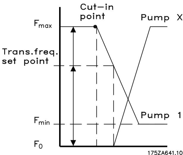
The opposite process occurs during destaging where a momentary pressure drop is avoided by increasing the speed of the adjustable speed pump. Therefore, set a transition frequency roughly half-way between minimum and maximum frequency.
