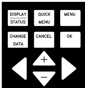
[DISPLAY/MODE] is used to change display modes or to return to the Display mode from either the Quick Menu or the Extend Menu mode.
