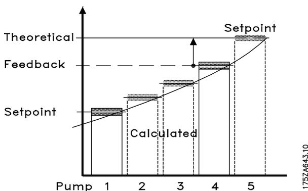
The range is determined by Quick Menu item 014 (parameter 413, *Minimum Feedback*) and Quick Menu item 05 (parameter 414, *Maximum Feedback*).
