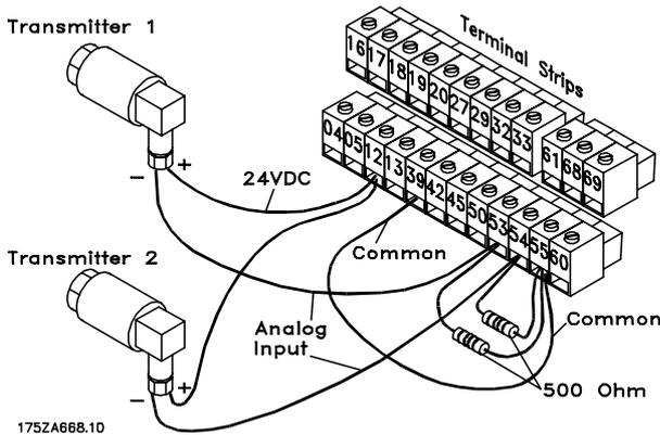
If the transmitter is capable of producing 10V at 20 mA, the value of the resistor to use is:
