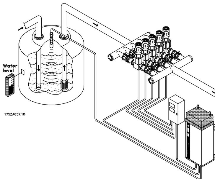
Level Control in Standard Cascade Control Mode
